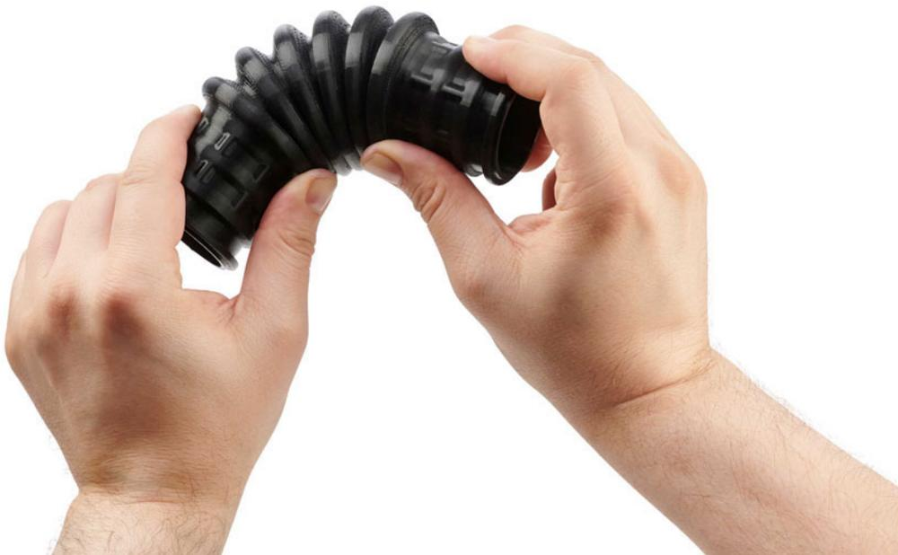
**TPU – Shore A – 92 hardness. Flexible Elastomer**
